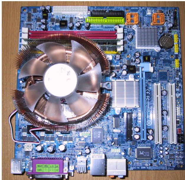
Illustration 3: Motherboard with AMD Athlon 64 X2 5200+ CPU and Cooler Installed
